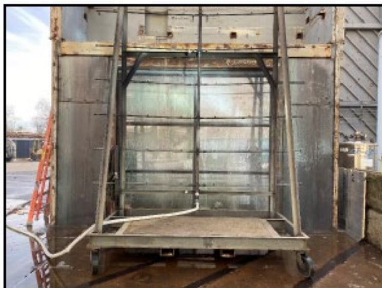
Photo No. 2 Exterior View During Static Water Penetration Testing @ 8.0 psf
